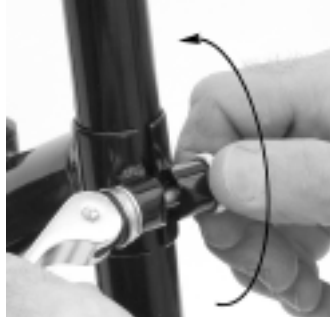
Figure 4d. Adjusting the QR clamp tension.
